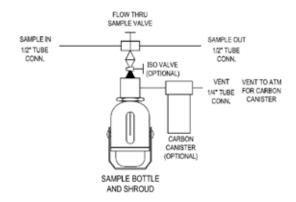
The MD - FlowThru System can be used for higher pressures and temperatures where a continuous flow loop is desired or viscous process is encountered.
