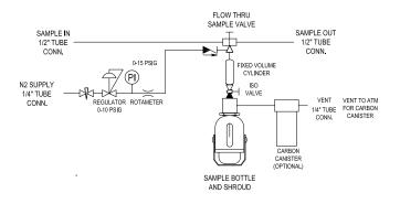
The MD Fixed Volume Sample System is designed to take a specified amount of sample in high pressure applications and a wide variety of viscosities.
