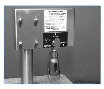
The MSD - Manual Continuous System features a threeway ball valve for traditional grab samples by rotating valve handle 180 degrees. The MSD Sample System is typically used for low pressure and temperature applications.
