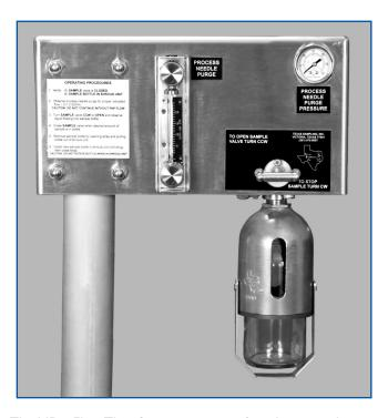
The MD - Flow Thru System consists of a robust sample valve that allows for continuous flow through a 1 / 2" orifice. The rising stem style sample valve allows the operator to control the flow of the sample being dispensed into the sample bottle. This system can be used for higher pressures and temperatures where a continuous flow loop is desired or viscous process is encountered. This sample valve is available in a variety of materials including chemical resistant plastics.
